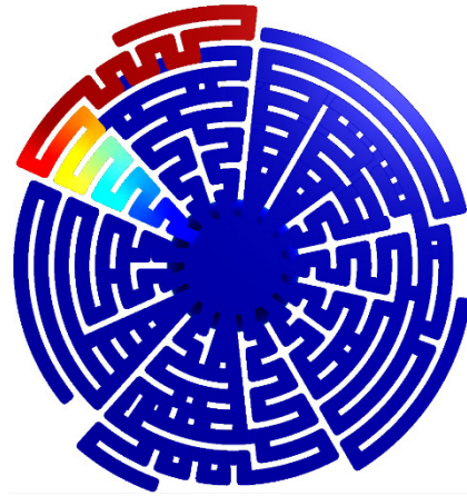
Figure 8 – Pressure distribution computed by finite element analysis for the first resonance at 620 Hz, showing that only one channel is excited. The second layer is in the background, explaining why the rendering of the channels geometry is sometimes altered.
