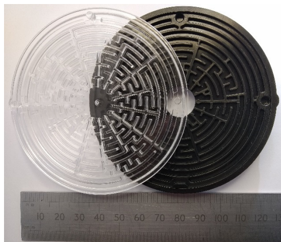
Figure 10 – Metamaterial absorber made with two injection molded parts. The overall thickness is only 11 mm.
